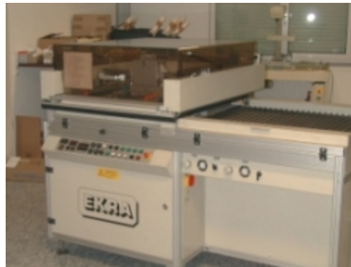
Photo 2: silk screen printing machine, Faber Electronics BV, Velp.
